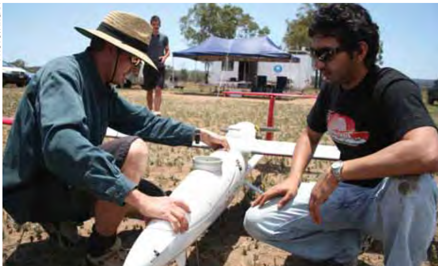
Australian Research Centre for Aerospace Automation (ARCAA) researchers Richard Glascock (left) and Pritesh Narayan set up spore traps on an unmanned aerial vehicle for the CRC project.
