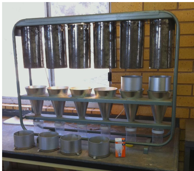
Figure 9. Tullgren funnels used for extracting insects from plant samples. Tests with wheat spiked with LGB adults demonstrated high levels of recovery over 48 hours.
