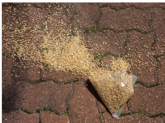
Figure 1. Press seal bags filled completely with seed (left), or paper bags with soil (right) did not maintain integrity when dropped 9m.
