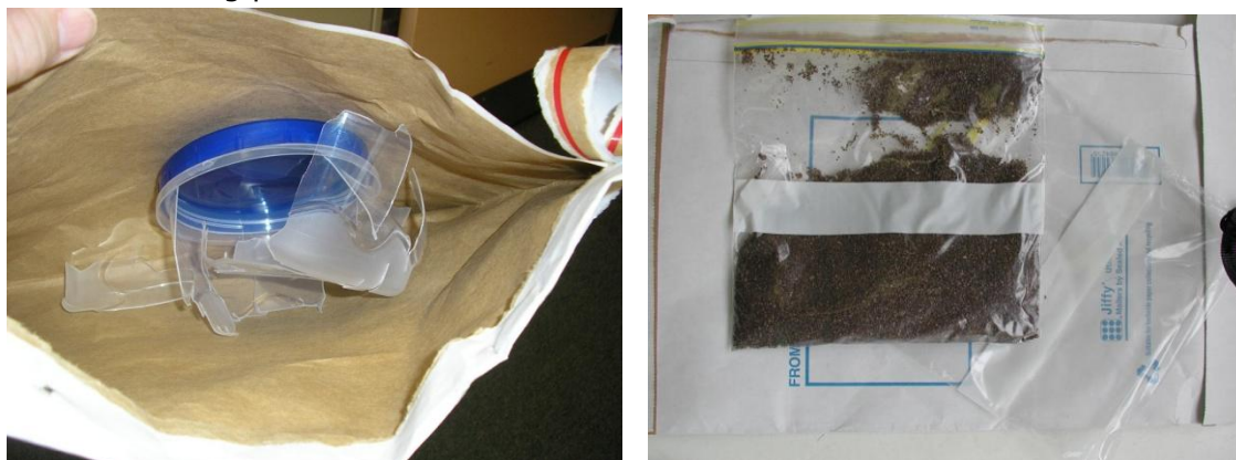
Figure 4. Plastic containers inside Tough bags did not survive postage while the Tough bag maintained integrity (Left). A small amount of soil leaked from primary press seal bag but was contained within the secondary press seal bag when posted in a Tough bag (right).
