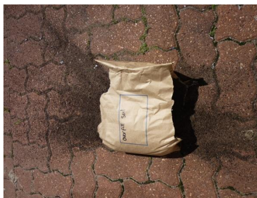
Figure 1. Press seal bags filled completely with seed (left), or paper bags with soil (right) did not maintain integrity when dropped 9m.
