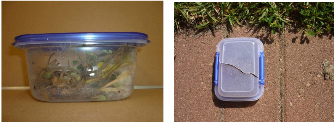
Figure 2. plastic containers dropped from 9m maintained integrity when used for light herbaceous material (left), but not with soil or seed (right).
